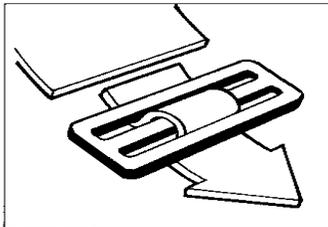
**STEP 1:** Insert strap through tightening buckle.
