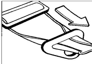
**STEP 2:** Pull strap to 8"-10" beyond buckle, fold edges and insert into mounting bracket.
