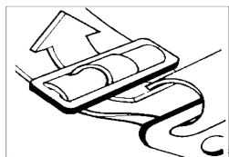
STEP 3: Fold back strap and re-insert through
