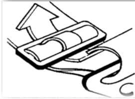
STEP 1: Insert strap through tightening buckle.
