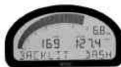
MoTeC's Advanced Dash Logger can be found in many Porsches racing in IMSA and Grand Am. This flexible dash, and configurable software can
