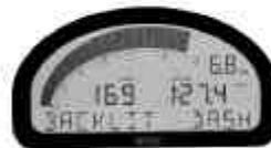
MoTeC's Advanced Dash Logger can be found in many Porsches racing in IMSA and Grand Am. This flexible dash, and configurable software can unlock the secrets of car setup and handling.
